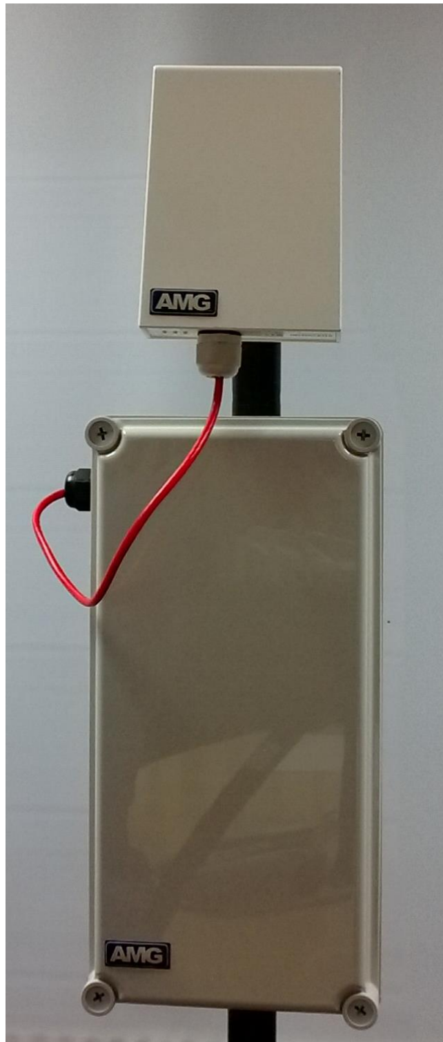
Radio and Encoder/Decoder housing mounted on the same pole.
