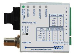
The **AMG5713** is a compact standalone one channel video transmit unit designed to transmit 1 video signal and transmit and receive 1 data signal plus 1 bi-directional alarm over one Singlemode optical fibre.
