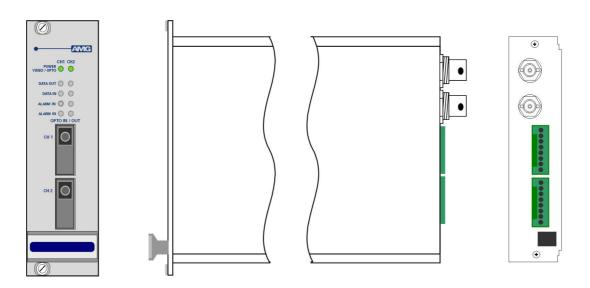
The **AMG5625R** is a **DUAL** rackmount system which provides two independent channels, each designed to transmit 1 video signals plus 2 Uni-directional alarms and transmit and receive 1 data signal over one Multimode optical fibre.
