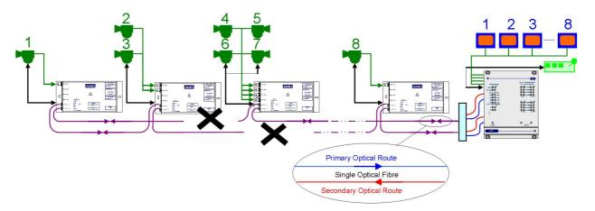
Note that where necessary repeaters can be added at nodes to increase the average distance between nodes.
