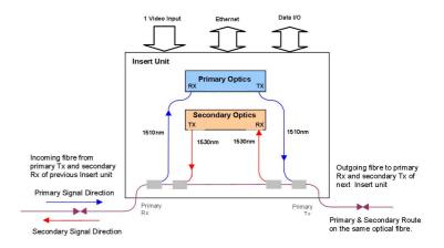
As each unit regenerates the optical signal of the same wavelength, the optical dynamic range between each optically connected node of the same wavelength is 22dB.
