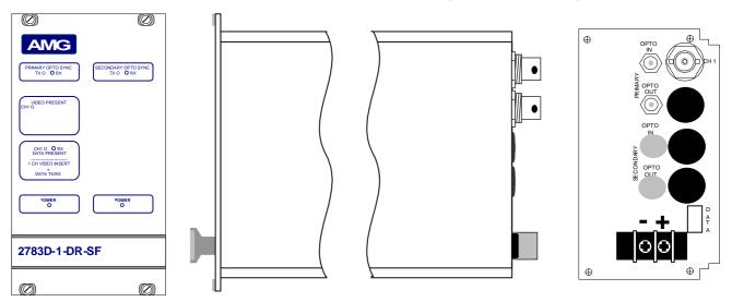
**AMG2783D-1-DR-SF** is a single channel video insert unit designed to transmit a video signal on to a single dual redundant optical fibre ring. It also provides a RS485/RS422 bi-directional data channel. The **AMG2783D-1-DR-SF** unit is supplied mounted in a basic subrack as shown below.
